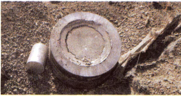
Figure 6. Depression formed from 200 mm diameter charge (front face).
