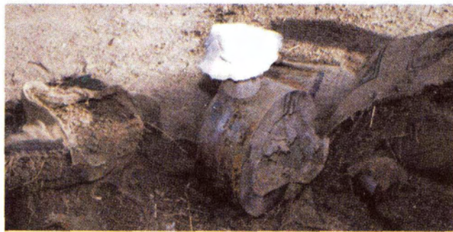
Figure 8. Scab from 150 mm diameter charge
