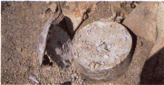
Figure 7. Multiple scabs from 200 mm diameter charge (rear face).
