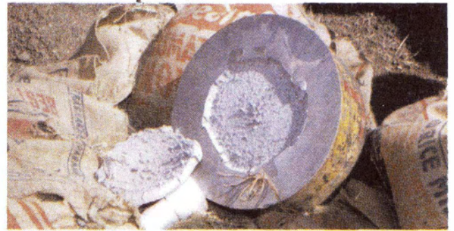
Figure 9. Scab from 100 mm diameter charge
