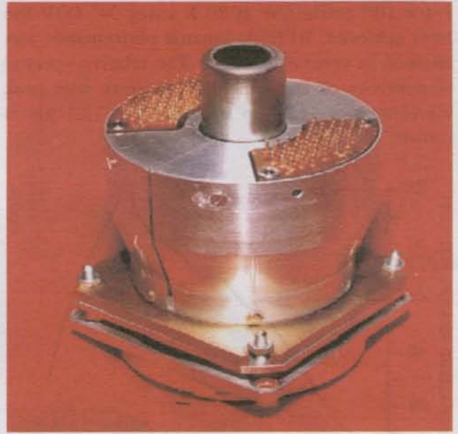
Figure 24(c). A 60-element photoconductive array as a packaged device.
