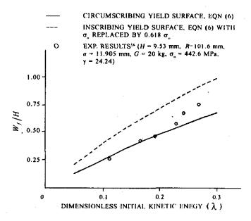
Figure 5. Comparison of the theoretical predictions of Eqn (6) with experimental results on fully clamped aluminium alloy circular plates struck by masses at the centre.
