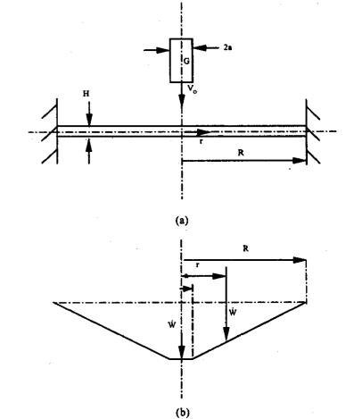
Figure 1. (a) Rigid cylindrical mass G striking a fully clamped circular plate and (b) axisymmetric transverse velocity profile at time t for the circular plate in Fig. 1(a).
