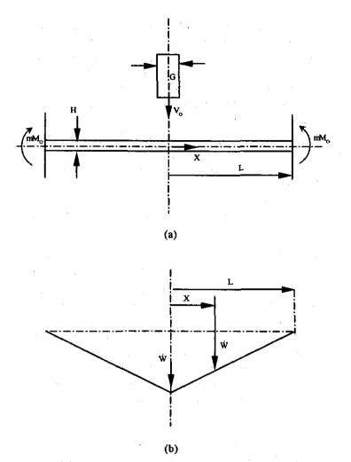
Figure 3. (a) Rigid mass G striking a square plate having a moment resistance  $(mM_0)$  around the outer supports (m = 0 and m = 1 give simply supportedand fully clamped cases, respectively) and (b) side view of pyramidal-shaped transverse velocity field at time t for the square plate in Fig. 3(a).
