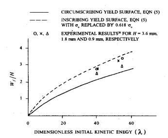
Figure 6. Comparison of the theoretical predictions of Eqn (5) with experimental results on fully clamped steel circular plates struck by a mass at the centre.
