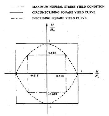
Figure 4. Yield conditions along the plastic hinge lines in the square plate in Fig. 3(a).
