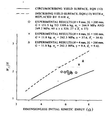
Figure 7. Comparison of the theoretical predictions of Eqn (13) with experimental results on fully clamped steel square plates struck by a mass at the centre.
