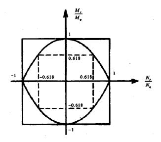
Figure 2. Uncoupled square, or limited interaction, yield condition for the circular plate in Fig. 1
