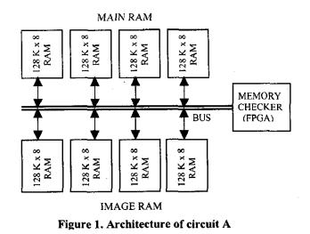
logic for data storage and retrieval is implemented in an FPGA chip. The same data is stored in the main RAM and image RAM. While it is read back, the data in the main and the image locations are compared. If any mismatch is detected, the processing logic will pass on the information to the CPU and onboard computer (OBC) will be switched to the redundant chain.
