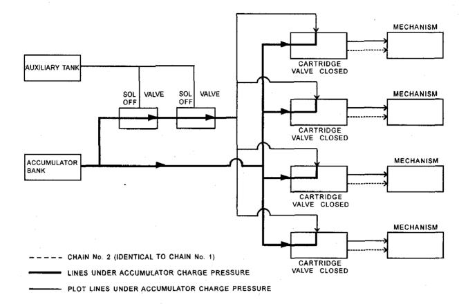
Figure 2. Schematic of hydraulic system
