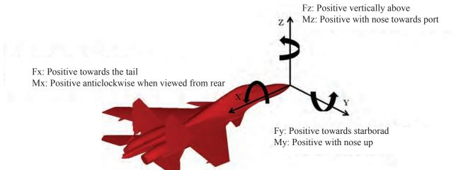
Figure 4. Sign convention for aerodynamic forces and moments.
