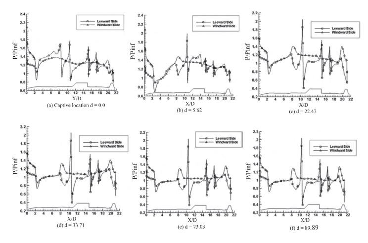
Figure 8. Pressure distribution on leeward and windward side of inboard missile (M = 1.2,  $\alpha = 10^{\circ}$ ).
