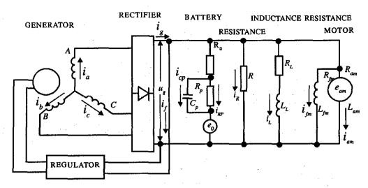
Figure 6. Schematic diagram of equivalent circuit of electrical system in military vehicle
