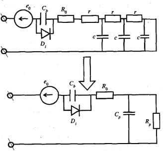
Figure 4. Equivalent circuit of the battery
