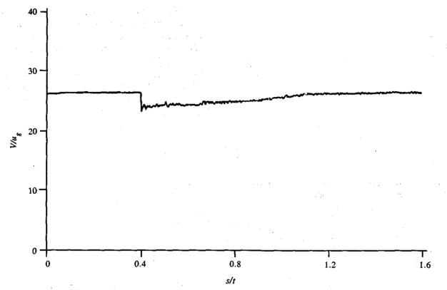
Figure 11. Surge measured in the combined generator-battery power supply
