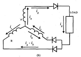
Figure 1. Functional mode of bridge rectifier
