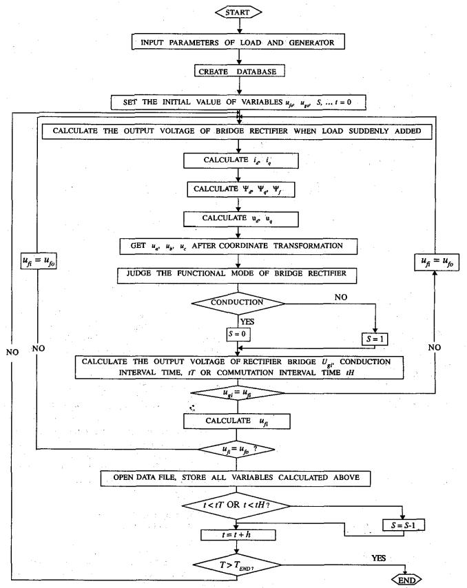
Figure 7. Program flowchart for calculation
