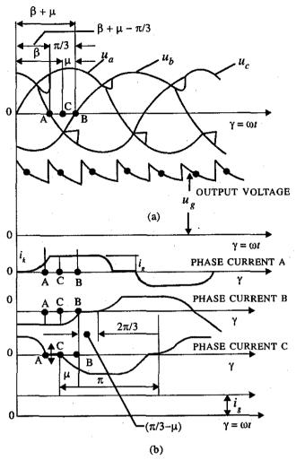
Figure 2. Relationship between (a) voltages and (b) currents.
