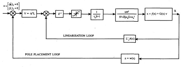
Figure 5. Feedback linearisation guidance law (Schematic)
