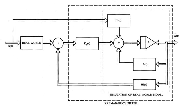
Figure 2. Structure of information processing by linear filtering techniques
