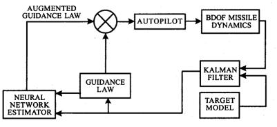
Figure 7. Schematic diagram of neural network-based guidance law
