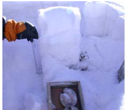
Figure 6. A column failed after few steps of loading.
