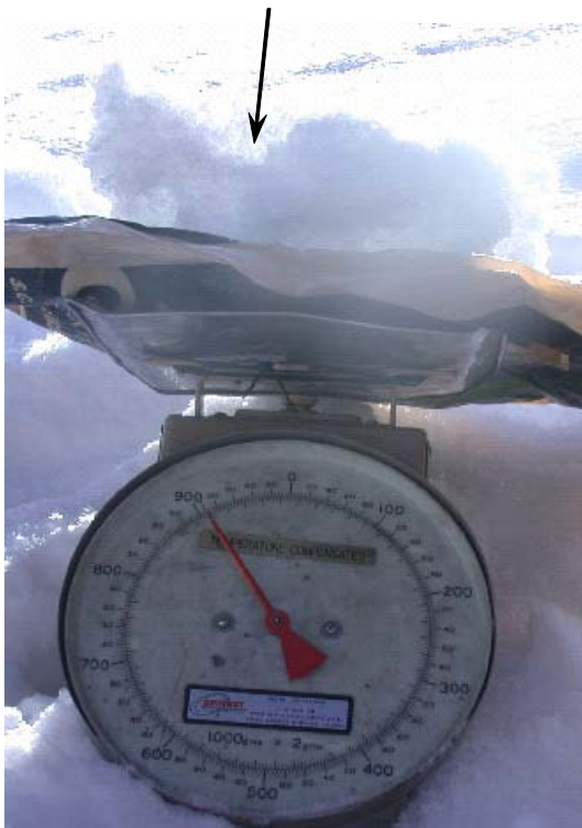
Figure 1. A snow block over the weighing machine for loading the snow columns but snow grains disintegrated in large amount during the preparation and weighing of snow block.
