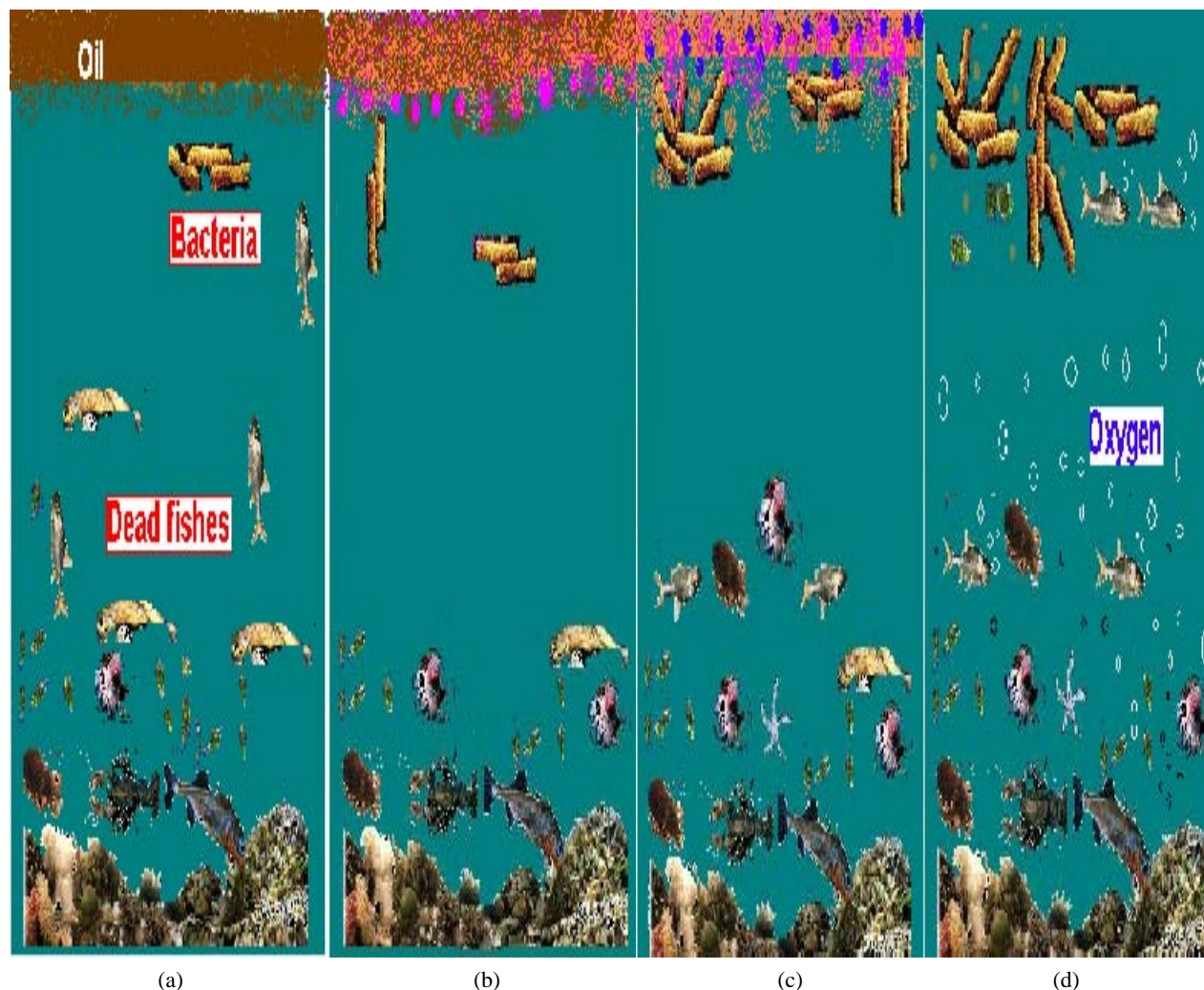
Figure 1. Schematic representation of bioremediation of floating oil in marine environment: (a) fuel oil pollution causing death of local flora and fauna, depletion of oxygen and light, (b) addition of bioemulsifier and nutrients facilitated emulsification of oil and growth of local oil utilizing bacteria, (c) addition of enriched consortium of oil-degrading bacteria along with bioemulsifier and nutrients facilitated fast emulsification, dispersion and degradation of pollutant oil, and (d) complete dispersion and degradation of oil achieved by bioremediation with nutrients, bioemulsifier and oil-degrading bacteria providing clean and healthy environment to marine organisms.
