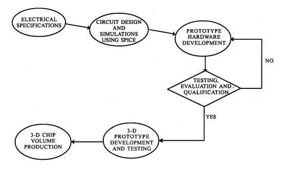
Figure 1. Flow diagram showing the 3-D MCM development
