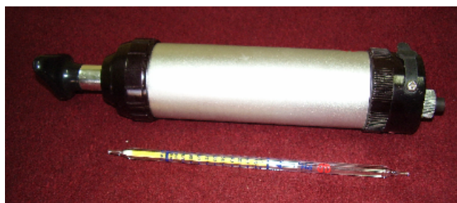
Figure 2. Sampling pump and phosphine detection tube.
