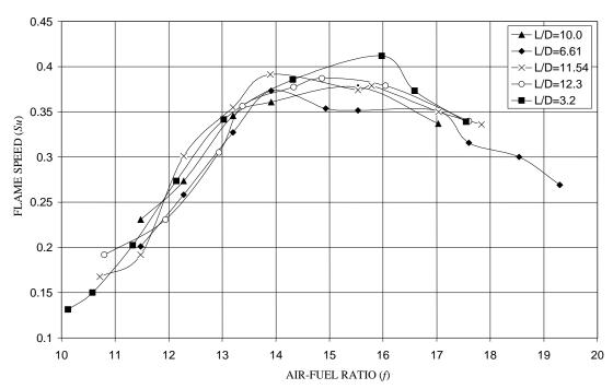
Figure 3. Variation of flame speeds with air-fuel ratio and different L/D ratios.
