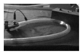
Figure 2. Premixed flame traveling in the heat-resistant tube of the test rig.
