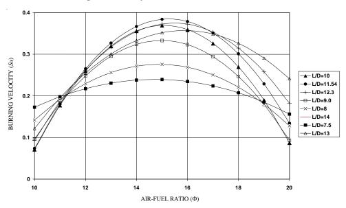
Figure 6. Design plot for various burner geometries.
