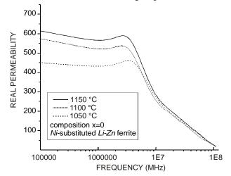
Figure 1. Real permeability (μ'<sub>s</sub>)/frequency of ferrite composition x=0, Li<sub>0.25</sub>Zn<sub>0.5</sub>-Mn<sub>0.1</sub>Fe<sub>2.15</sub>O<sub>4</sub> ferrite material sintered at 1050 °C, 1100 °C, and 1150 °C.
