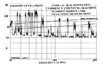
Figure 10.Peak Noise (dBpW) versus Frequency (MHz). Noise radiated by the currency counting machine (No Ferrite used to suppress the electromagnetic noise).
