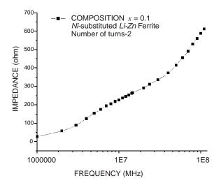
Figure 3. Impedence versus frequency of Ni–substituted Li-Zn ferrite  $Li_{0.25-x/4}Zn_{0.5-x/2}Ni_xMn_{0.1}Fe_{2.15-x/4}O_4$  where x = 0.1.
