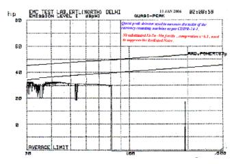
Figure 12. Quasi peak noise (dBpW) versus frequency (MHz). Radiated noise of currency counting machine measured by the quasi peak detector (*Ni*-substituted *Li-Zn-Mn* Ferrite composition x = 0.1 used to suppress the noise)
