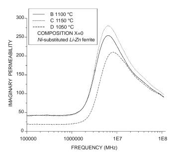
Figure 2. Imaginary permeability  $(\mu''_s)/\text{frequency of ferrite}$ composition x=0,  $Li_{0.25}Zn_{0.5}-Mn_{0.1}Fe_{2.15}O_4$ , ferrite material sintered at 1050 °C, 1100 °C, and 1150 °C.
