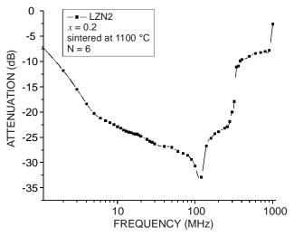
Figure 5. Insertion loss versus frequency for the composition x = 0.2, number of turns n = 6.
