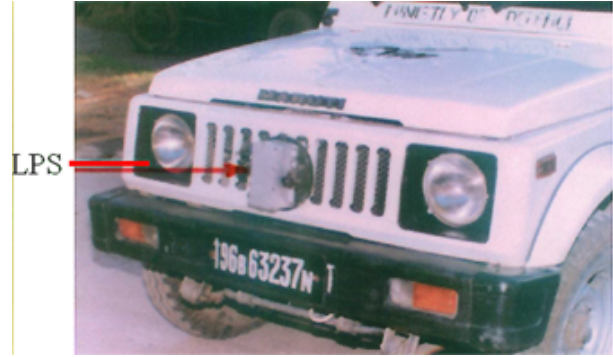
Figure 4. Laser proximity sensor mounted on a vehicle for dynamic trials.
