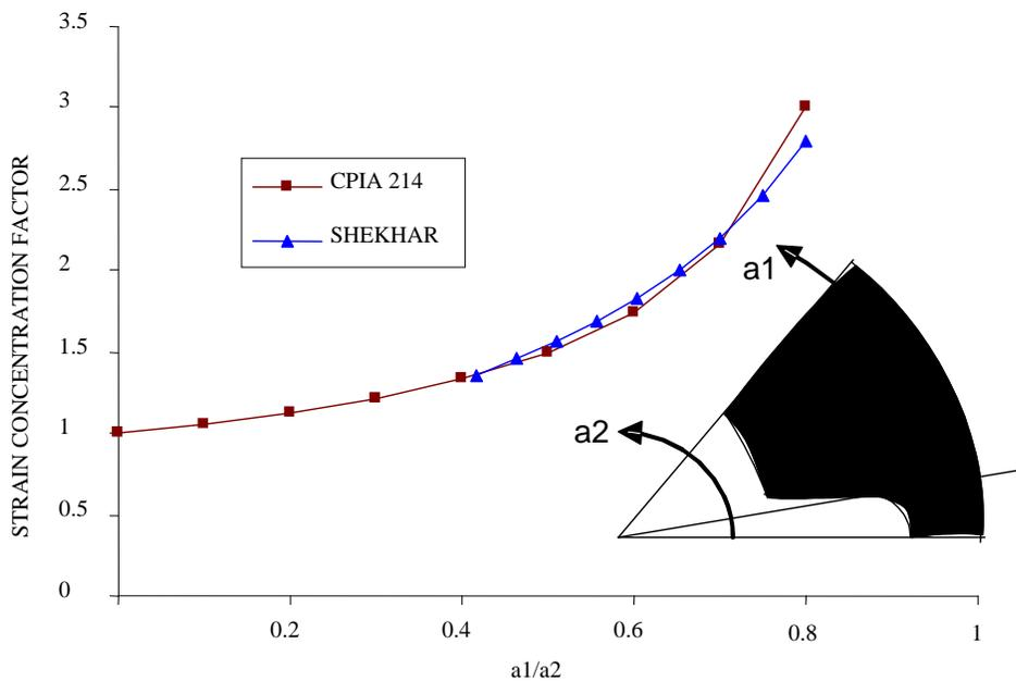
Figure 8. Comparison of strain concentration factors.
