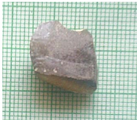
Figure 2. Grown PZN-PT (91-9) single crystal by bottom-supported flux Bridgman method.
