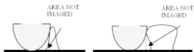
Figure 7. Tip dilation of structural features on the surfaces.
