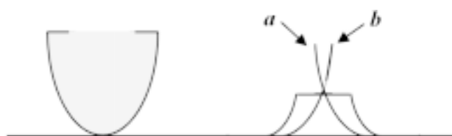
Figure 11. Erosion process of an image feature with a probe geometry that is too blunt. Erosion of right side of the image feature produces surface 'a' and erosion of left side of the image feature produces surface 'b'.
