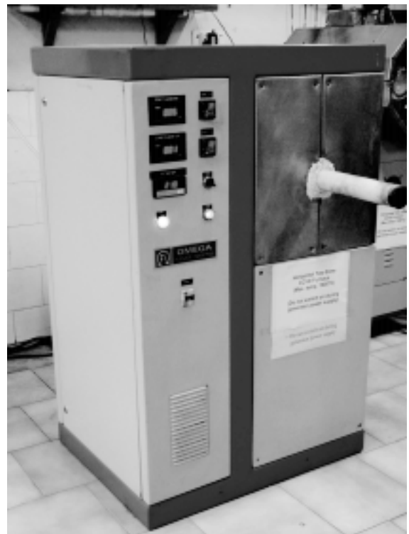
Figure 3(d). High temperature catalytic CCVD furnace (1600 °C).
