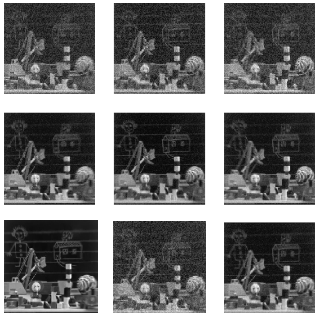
Figure 4. Top row shows the image affected by random noise. Second row shows images after noise suppression after filtering. Bottom row shows (left to right) fusion of clean image, noisy images and filtered noisy images. The RMS fusion rule was used for all.
