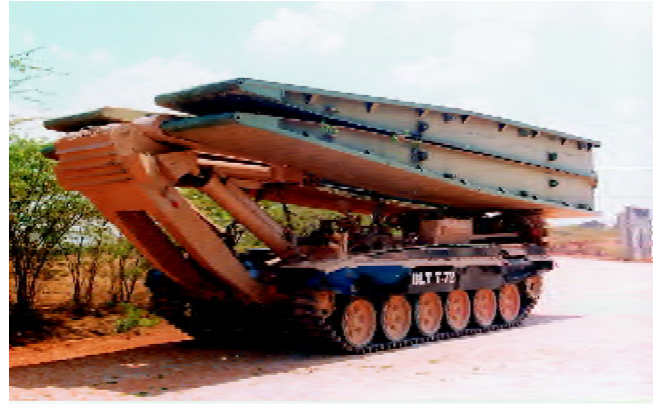
Figure 1. Typical bridge layer tank-T72.
