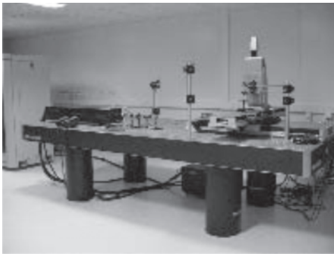
Figure 5. Microstereolithography (MSL) setup at NPOL.
