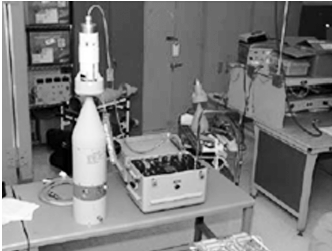
Figure 4. Laser seeker head being tested with MRTS.
