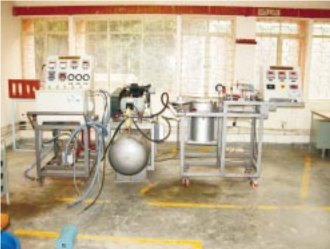
Figure 3. Reducer and breathing bag test facility MK-I.
