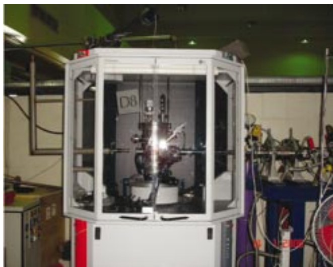
Figure 9. A view of in-situ X-ray diffractometer in the beam line. The chamber has a port to connect to the accelerator beam line. The chamber also has two Kapton (polyimide) windows for the entry and exit of the incident and diffracted X-rays respectively.
