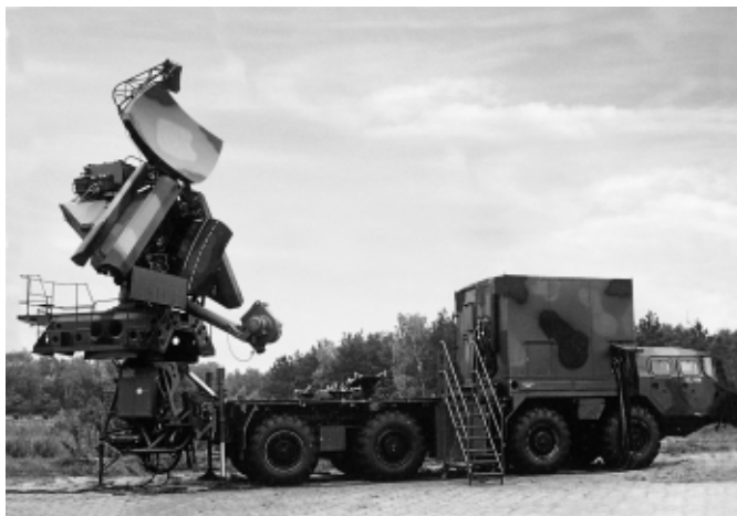
Figure 7. (WZE S.A. photo) Rocket homing station (NEWA SC) of (SA-3 SC) system.
