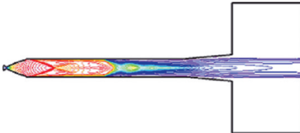
Figure 21. Mach contours inside HAT facility.
