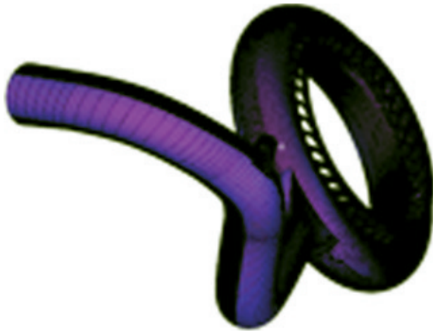
Figure 28. Computational grid for integrated analysis.
