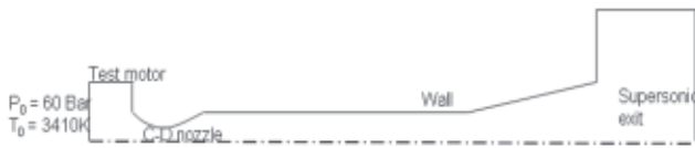
Figure 19. Computational domain for HAT facility.
