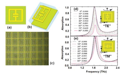
Figure 8. Flexible wide angle THz absorber and numerical calculations for high absorption over a wide range of angles of incidence for both TE and TM radiation<sup>14</sup>.
