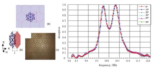
Figure 5. Bandwidth enhanced double resonance metamaterial absorber<sup>11</sup>.
