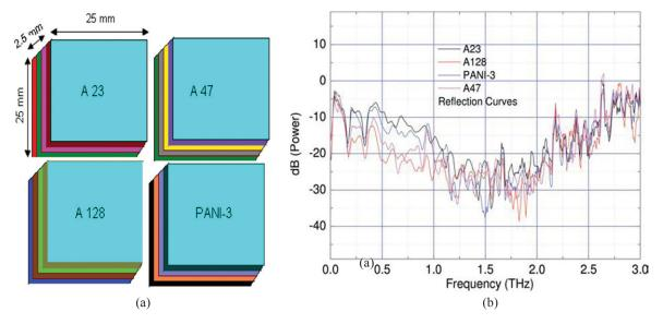
Figure 9. Schematic of fabricated structures (a) reflection loss measurements and (b) polymeric coating in THz region<sup>16</sup>.
