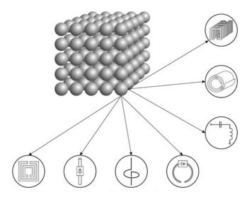
Figure 1. Illustration of metamaterial concept in terms of conventional materials<sup>3</sup>.
