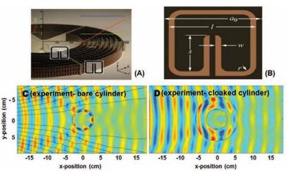
Figure 3. First experimental demonstration of cloaking at 8.5 GHz<sup>8</sup>.
