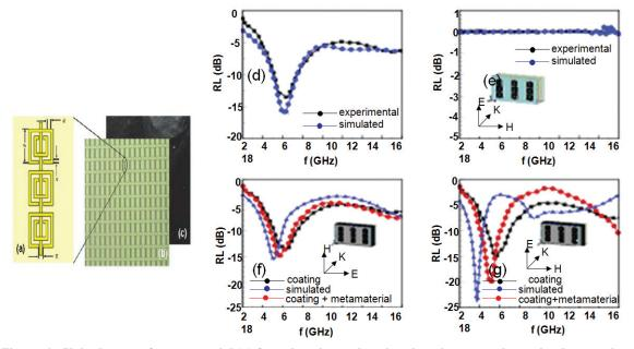
Figure 6. Unit element of metamaterial (a) for enhancing and tuning the microwave absorption by covering a single metamaterial layer (b) on CIPC (c) and observed results<sup>12</sup>.
