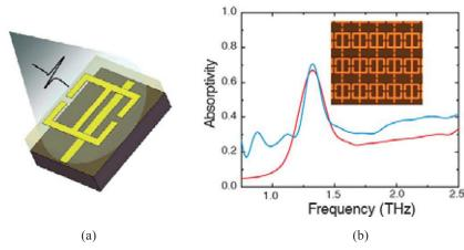
Figure 7. Metamaterial based absorbers for terahertz frequency region<sup>13</sup>.
