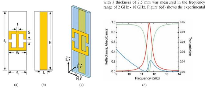
Figure 4. (a) Electric resonator and (b) cut wire components of unit element (c) unit element with dielectric spacer and direction of wave propagation, (d) simulated pattern for reflectance, absorbance and transmission<sup>9</sup>.
