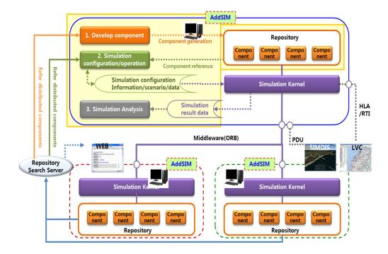
Figure 9. Operational concept of AddSIM (notional).
