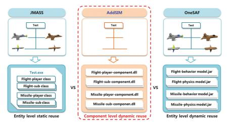
Figure 6. Comparison of reuse methodology among JMASS, AddSIM and OneSAF.
