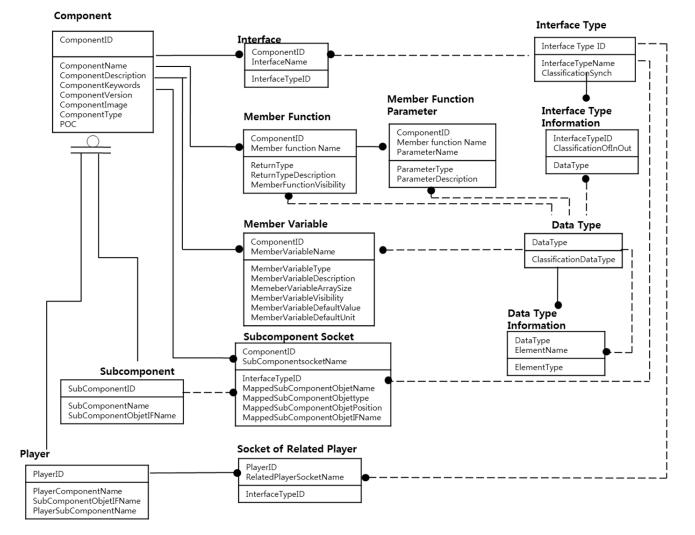
Figure 5. A meta-model in AddSIM.
