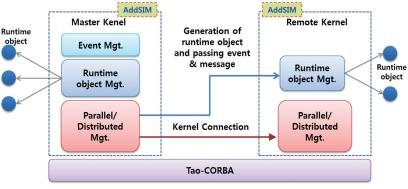
Figure 8. Operation mechanism of distributed processing.
