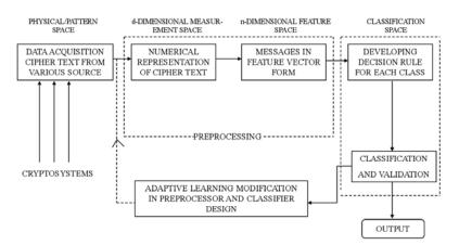
Figure 3. Block diagram of a crypto-system identifier.
