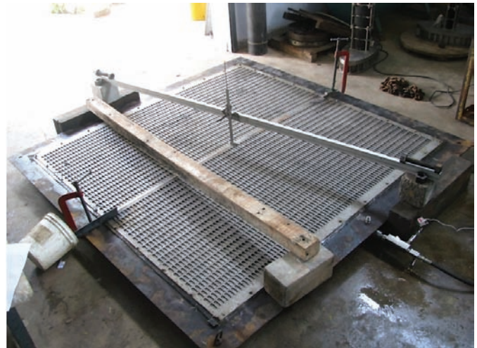
Figure 3. Experimental setup for load deflection of perforated plate with lining.
