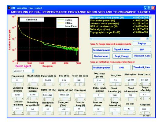
Panel 2. Graphical user display panel developed for DIAL system modelling.
