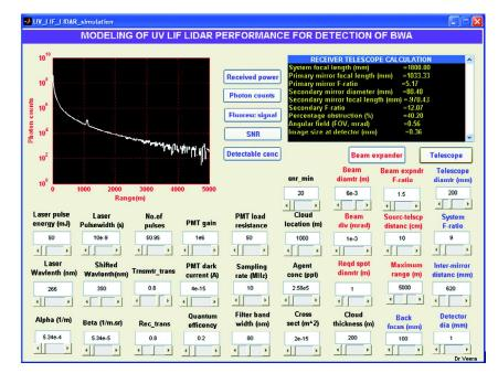
Panel 3. Graphical user interface display panel developed for LIF LIDAR system modelling.
