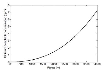
Figure 3. Minimum detectable concentration versus range computed for tabun agent using DIAL technique.
