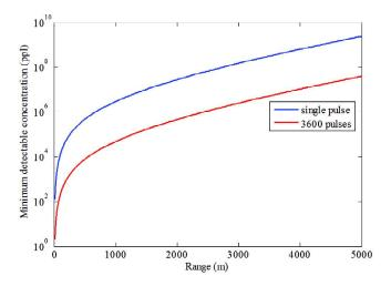
Figure 5. The minimum detectable concentration versus range computed for fluorescence LIDAR for transmission of single pulse and the average of 3600 pulses.
