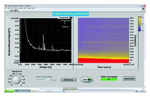
Panel 1. LIDAR controller and data acquisition display panel. The backscattered signals shows the presence of multiple clouds at distances of 3.5–3.9 km.
