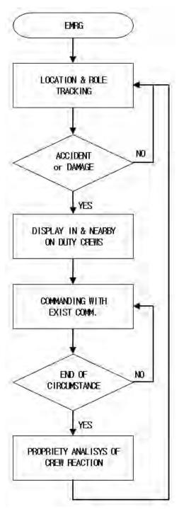
Figure 1. Flow chart of a damage control concept using crew member location tracking.
