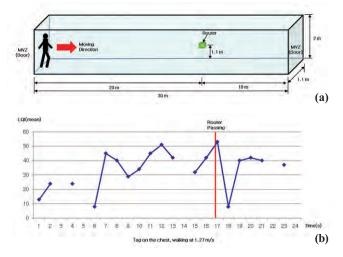
Figure 3. Test environment and initial experiment result: (a) test environment of location tracking, (b) an example of walking speed ZigBee tag experiment results without mediation.
