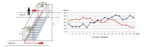
Figure 5. Experimental results of moving ZigBee tags traversing between decks.
