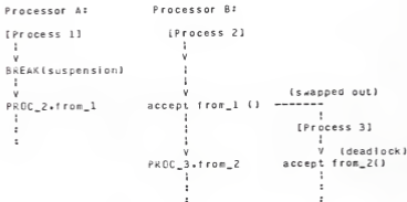
Figure 5.1a: Deadlock in a multiple processors system
