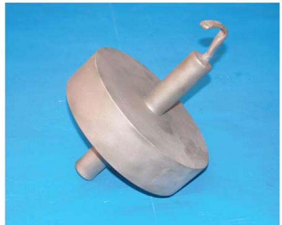
Figure 6. Capsules of the rotor before hot isostatic pressing.
