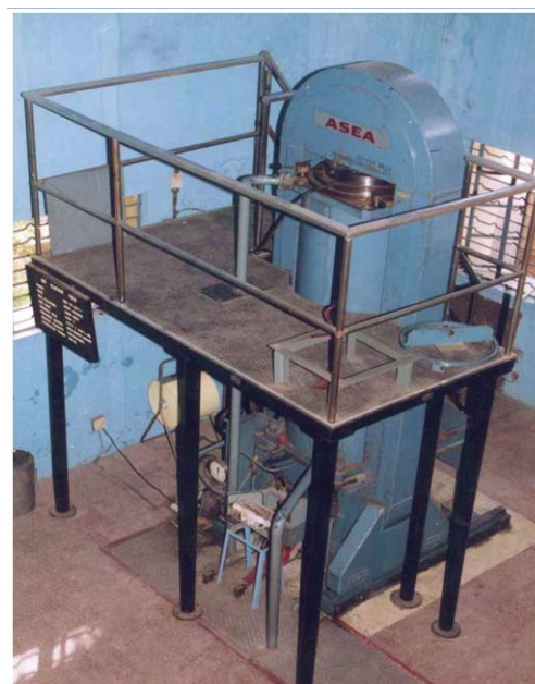
Figure 1. Hot isostatic pressing facility at DMRL.
