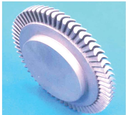
Figure 8. HIPed superalloy 718 integral turbine rotor.
