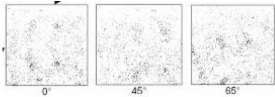
Figure 4. Orientations measurement from the early stage of recrystallisation ( 400^\circ\text{C} ). The 0^\circ , 45^\circ , and 65^\circ constant \phi_2 sections (of orientation distribution function) of grain orientation obtained from EBSD experiments. No preference of the ideal orientations (Cube, Cu , Bs , and S ) is observed during nucleation.
