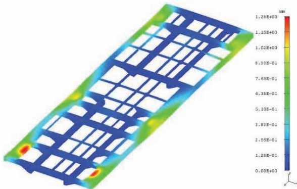
Figure 7. Deflection: Type-I loading.
