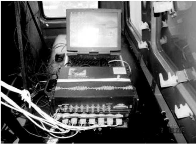
Figure 14. Data acquisition system-Wavebook 512 with strain gauge module WBK-16.
