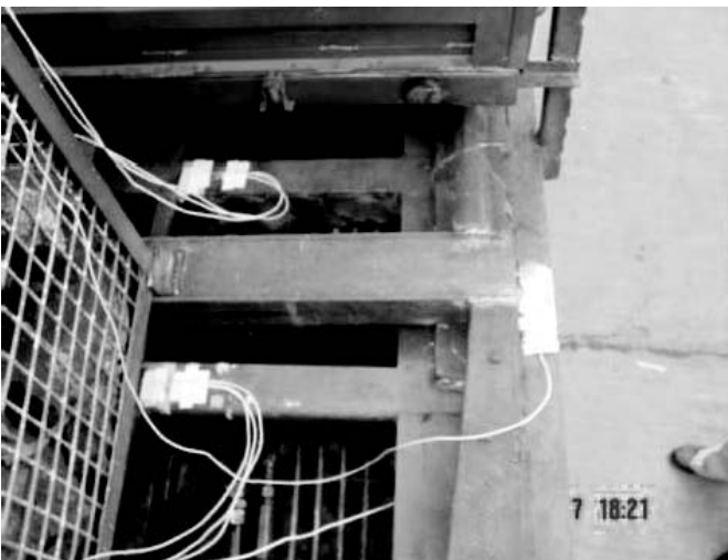
Figures 15. Location of strain gauges on CM-5 and CM-6.
