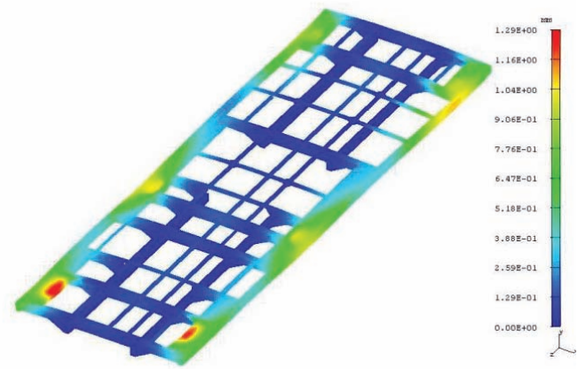
Figure 12. Deflection: Type-I with mast moment.
