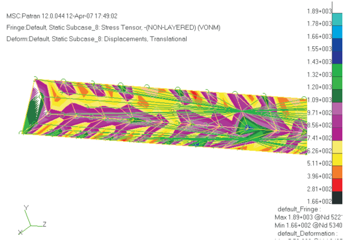
Figure 12. Visual FEM result for stress distribution of weldment.
