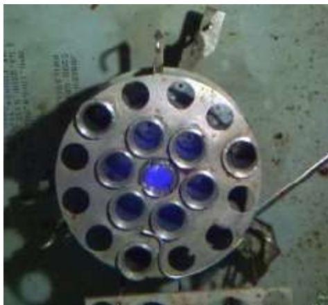
Figure 3-5 Image of the ^{60}\text{Co} source used to irradiate the samples. Photo courtesy of Cory D. Cress, U.S. Naval Research Laboratory.
