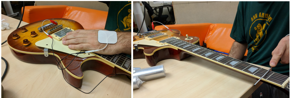
Figure 6.2: Testing a TENS unit on a standard electric guitar, and with conductive materials
