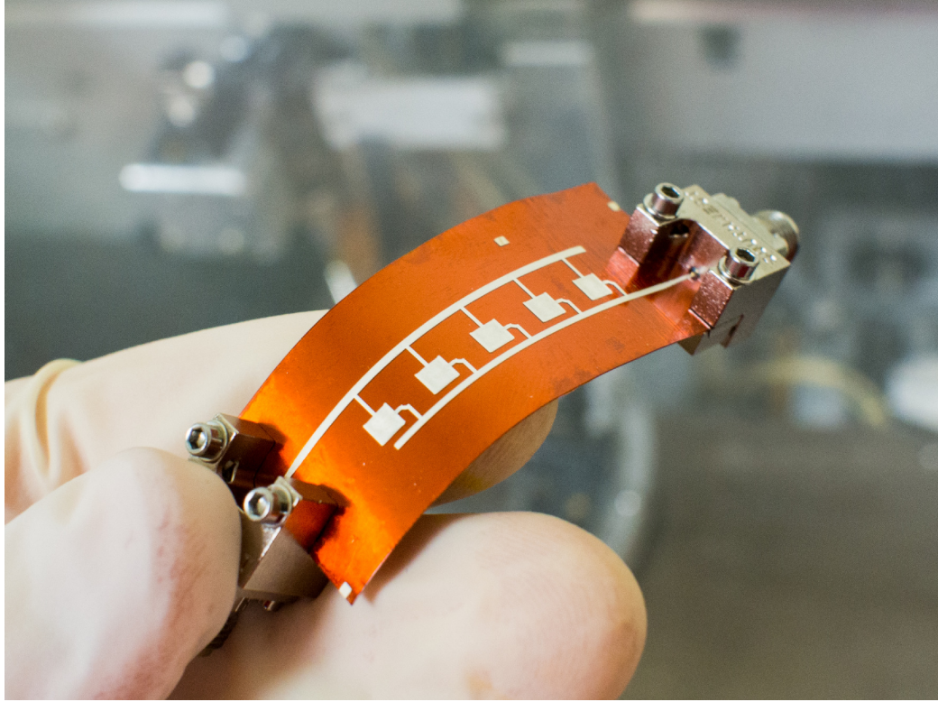
Figure 3.2: Inkjet-printed flexible linear antenna array
