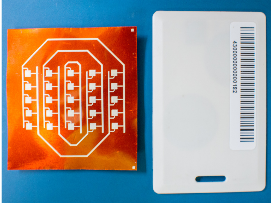
Figure 3.5: Inkjet-printed flexible Van-Atta reflectarray prototype, next to a standard "credit-card" size RFID tag package
