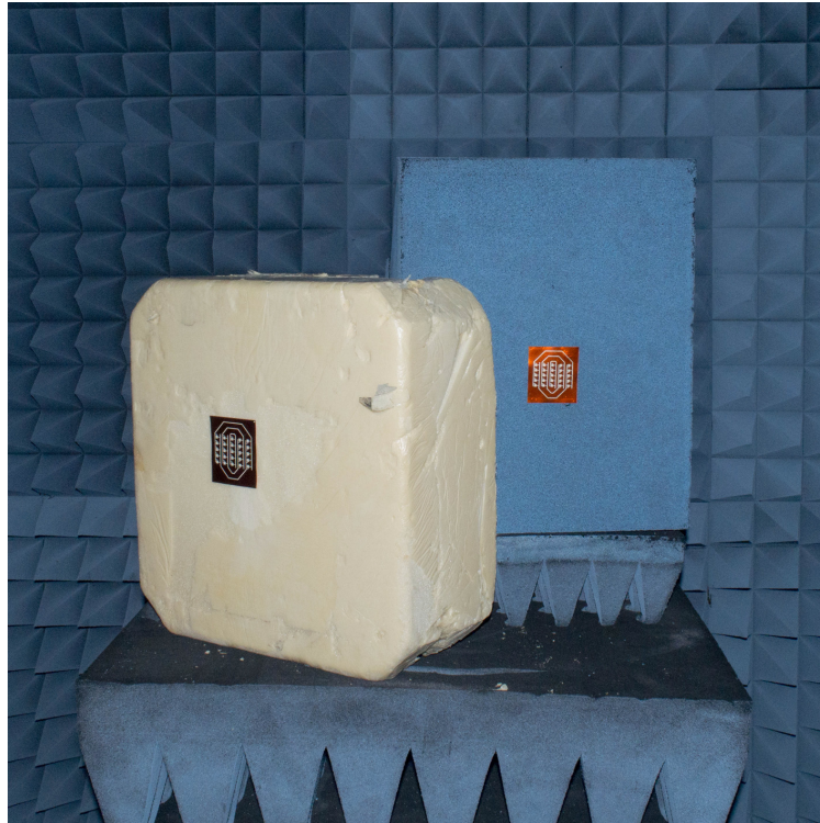
Figure 3.12: Target measurement configuration for dual-tag detection demonstration
