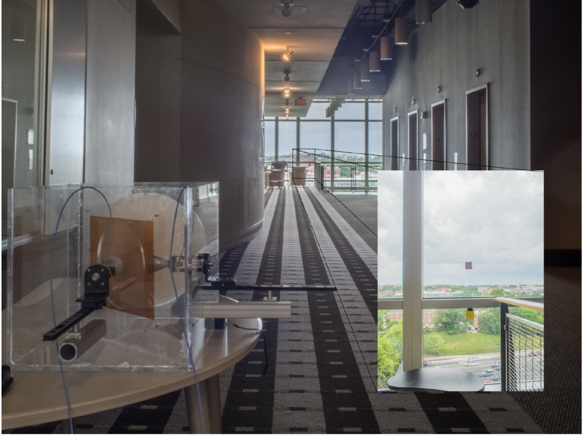
Figure 3.15: Measurement configuration at an interrogation range of 30.5 m
