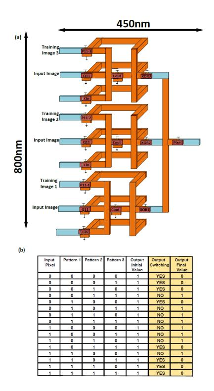
Figure 31: (a) Comparator-first pixel detector schematic. (b) The truth table with the detailed operation of the circuit.
