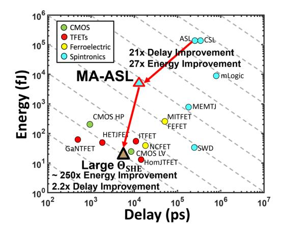
Figure 77: Delay and energy comparison of the MASO device with various spintronic, CMOS, and TFET devices. Compared to MA-ASL, the MASO device operates with  $2.2 \times$  and  $250 \times$  lower delay and energy dissipation, respectively. Compared to CMOS, device operates with lower delay-energy product.
