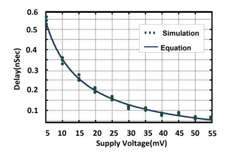
Figure 26: Switching delay variation versus the supply voltage. Each voltage is simulated three times to verify the results.
