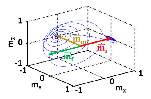
Figure 72: First, the orientation of Magnet 2, rotates by  $90^0$  from  $\vec{m}_i$  to  $\vec{m}_m$  using magnetostrictive switching; then, it reorients by  $90^0$  from  $\vec{m}_m$  to  $\vec{m}_f$  using SHE.
