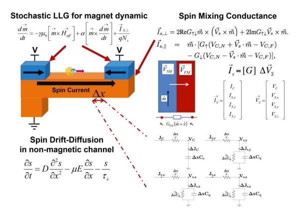
Figure 8: To model the physics of the all-spin logic device, magnetization dynamics, spin mixing conductance, and spin-drift diffusion in the channel are taken into account [78].
