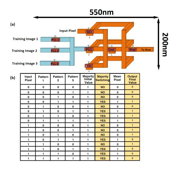
Figure 30: (a) Standard single pixel detector schematic. (b) The truth table with the detailed operation of the circuit.
