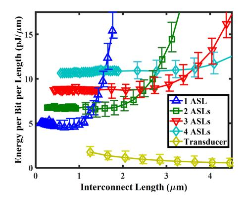
Figure 46: Energy dissipation per unit length of the ASL repeaters is compared to that of the proposed spintronic interconnect. The dissipated energy of the proposed interconnect is lower than that of repeaters even for  $L_{Int}$  as small as 1.25 µm.
