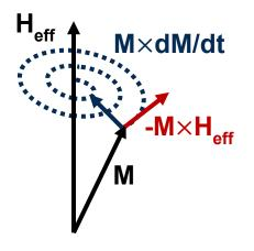
Figure 12: LLG equation describes the magnetization dynamics. The corresponding vectors to the terms of LLG equation are represented in this figure.
