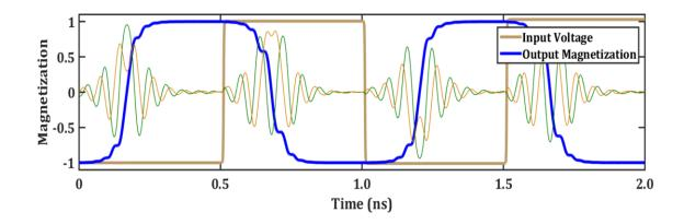
Figure 11: Transient Response of an all-spin logic device. In this simulation, the input magnet is assumed to be oriented in the +X direction. By applying a negative voltage, the device acts as a buffer, while by applying a positive voltage, the device acts as an inverter.
