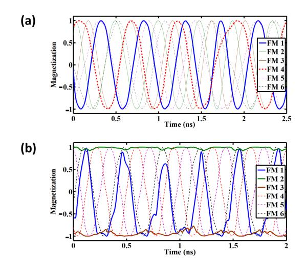
Figure 22: The voltage applied to the magnets of the ring 1 is 35 mV. In (a), the voltage applied to the magnets of the ring 2 is 10 mV higher than the voltage applied to the ring 1, while in (b), the voltage applied to the ring 2 is 20 mV higher than the voltage applied to the ring 1.
