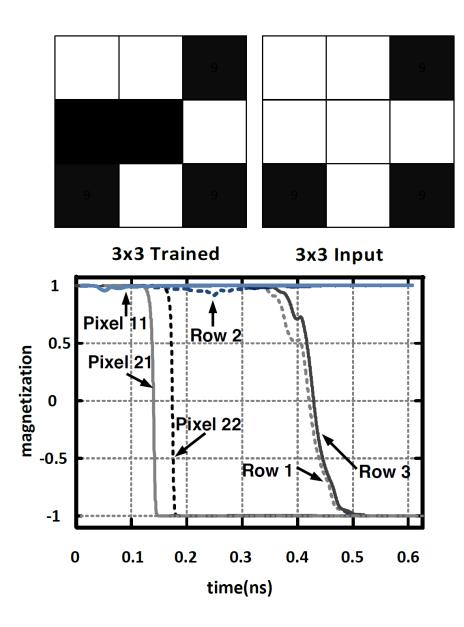
Figure 33: Using a single smart detector cell, we can compare these  $3 \times 3$  pixel images. The waveforms of the comparators and majority gates (bottom).
