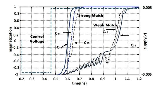
Figure 37: The switching delay of output magnetization in last stage represents the similarity of input data and pattern data.
