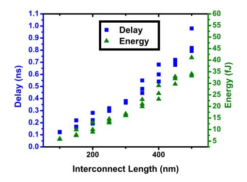
Figure 14: Delay and energy dissipation vs channel (channel) length of an ASL gate.
