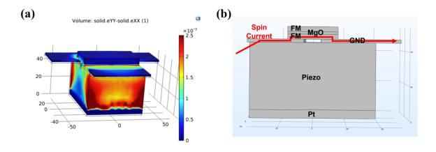
Figure 61: (a) Transferred strain to the magnet is 800 ppm, lower than that to an MA-ASL magnet; however, the transferred strain is enough to rotate the magnetization. (b) shows the path of applied spin current through the output magnet to ground.
