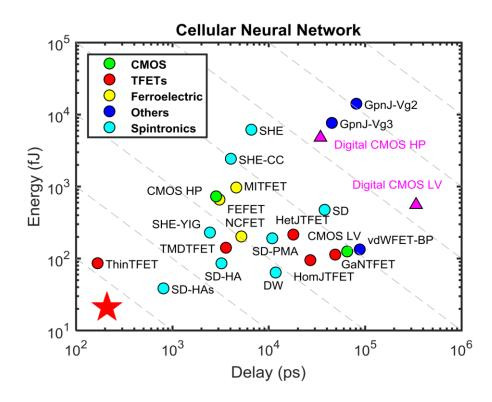
Figure 78: Energy versus delay per memory association operation using CNN for a variety of charge- and spin-based devices, where the red star indicates the preferred corner [32].
