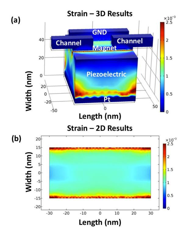
Figure 51: Generated strain is simulated using a COMSOL model developed from the piezoelectric parameters of PMN-PT [144]. Results shown for (a) the device and (b) the cross-section of the magnet demonstrate that the net strain of 1200 ppm will be transferred to the magnet.
