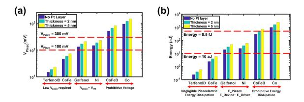
Figure 57: (a) voltage and (b) energy required to transfer a net strain of 1200 ppm to the magnetic layer. Simulations are done for various magnetic materials, in which Terfenol-D demonstrated lowest required voltage and energy dissipation for transferring strain. Moreover, the figure compares the transferred strain for various piezoelectric thickness values.
