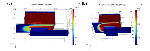
Figure 74: COMSOL simulations are done to measure the amount of the transferred strain for W as shown in (a) and Pt as shown in (b).
