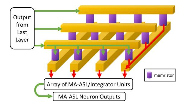
Figure 64: Memristive cross-bar network. The cross-bar array sums together the input currents, abbreviating the number of magnets needed for the output neurons [166].
