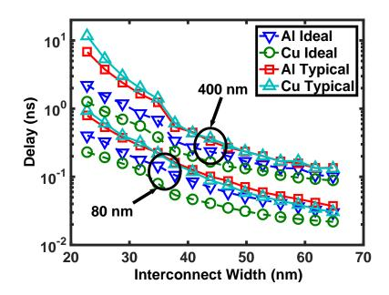
Figure 17: Delay versus channel width for 80 nm and 400 nm long channel.
