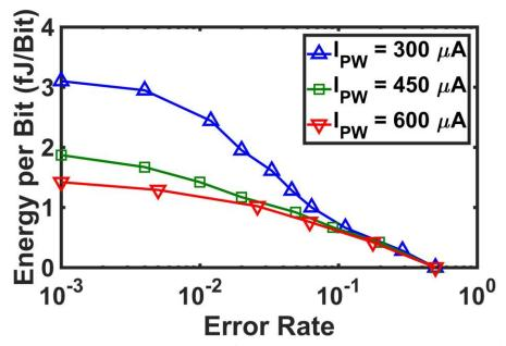
Figure 55: Increasing the amplitude of the pulse current, lowers the required pulse width to reach to the same error rate in an MA-ASL inverter; thus, as pulse amplitude increases, lower energy is required to reach to the same error rate. However, the amplitude of the pulse current cannot exceed certain maximum limits due to electromigration.
