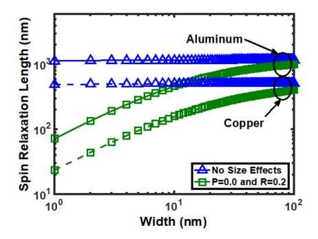
Figure 15: Spin Relaxation versus channel Width [2]. Size effects cause the spin relaxation length to decrease with decreasing channel width. For the no size effect case, spin relaxation length is independent of channel width.
