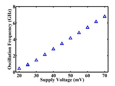
Figure 20: Oscillation frequency versus supply voltage. The oscillation frequency increases linearly with increasing the supply voltage.
