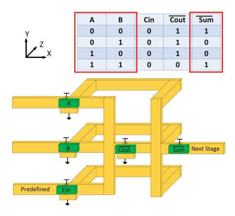
Figure 28: 1-bit full adder used as XNOR. In the 2D implementation of this work, X and Y wires are in-plane metal wires and connections along the Z axis are vias.
