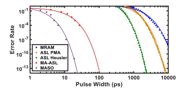
Figure 76: Write error statistics of the MASO device vs. the ASL device, the MA-ASL device, and the STT-MRAM [30], [72], [130], [222].
