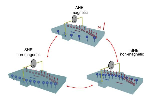
Figure 4: Illustration of spin-dependent Hall effects used in spin current generation and detection. In the SHE, an unpolarized charge current generates a transverse spin current, while in the ISHE, a spin current generates a transverse charge current. In the anomalous Hall effect (AHE), a charge current generates a transverse charge current [58].
