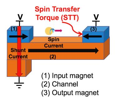
Figure 10: ASL consists of two magnets connected by a non-magnetic channel. Injected spin current from Input magnet to the channel diffuses along the channel and applies a torque to the output magnet, which if strong enough, switches the output magnet.
