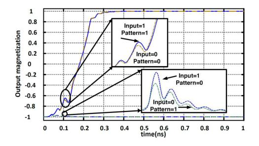
Figure 29: Simulated output waveforms of XNOR gate
