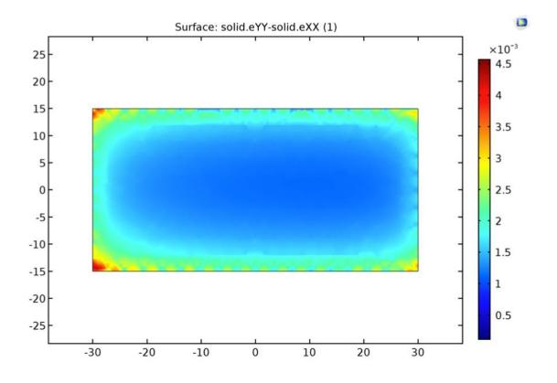
Figure 73: Transferred strain to the magnet is simulated using COMSOL, and the results are shown for the cross-section of the magnet.
