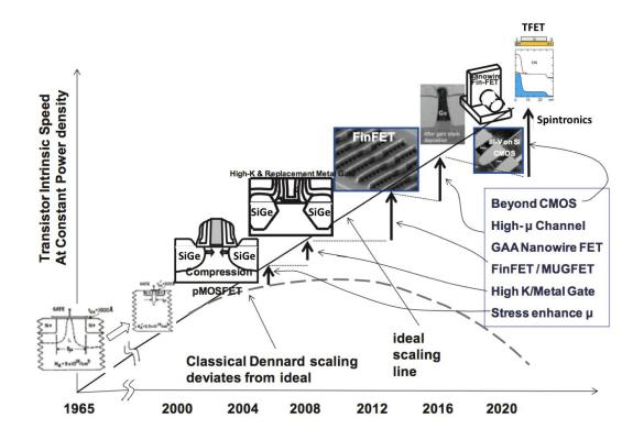
Figure 1: To improve the performance of FET transistors, various technologies are investigated over the past five decades.
