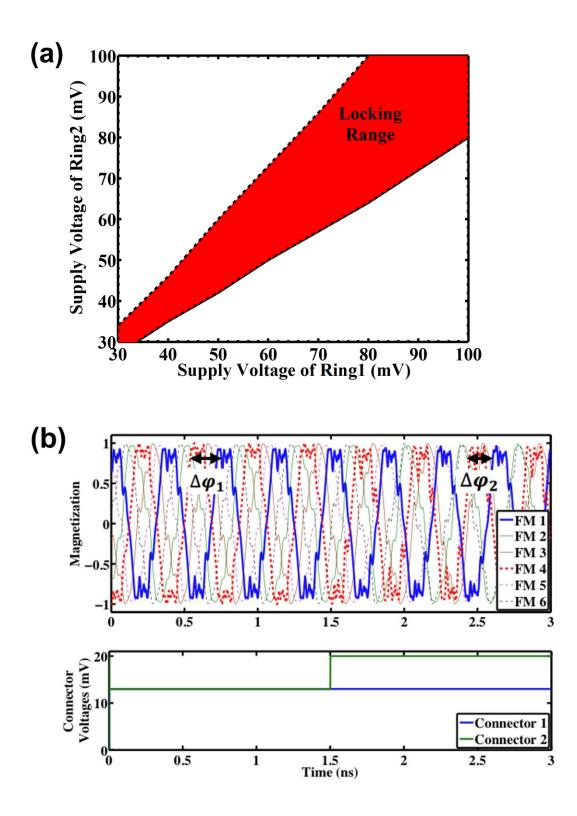
Figure 23: (a) The supply voltage applied to the ASL connector 2 is changed from 12.5 mV to 20 mV. As a result, the phase shift of the two rings is changed from  $\Delta\phi_1$  to  $\Delta\phi_2$  in which  $\Delta\phi_1 > \Delta\phi_2$ . (b) Locking range of the ASL coupled oscillator. The shaded
