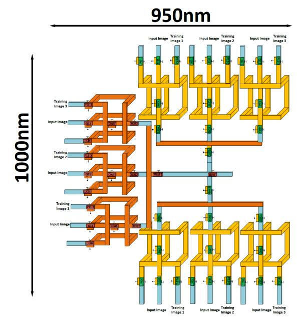
Figure 32: Structure of the unit smart detector cell.
