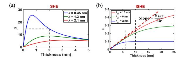
Figure 68: MATLAB simulations are done to measure the efficiency of the spin to charge and charge to spin conversion in the device. Based on the results, maximum spin to charge conversion is achieved by maximizing the thickness of the metallic layer, while the maximum charge to spin conversion efficiency is achieved by minimizing the thickness of the metallic layer.
