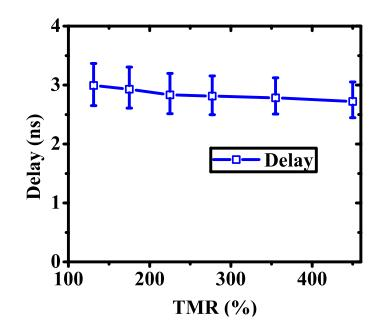
Figure 49: As TMR increases, the voltage swing at node  $V_N$  of Figure 43 becomes larger; hence, the delay becomes smaller. However, the voltage swing is relatively large even for TMR values as low as 125%, and the improvement in switching delay by increasing TMR is limited to less than 10%.
