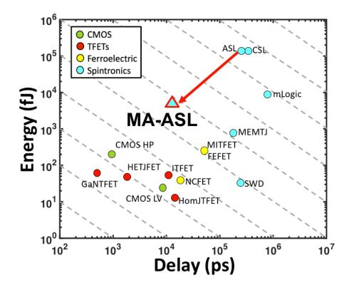
Figure 54: Energy dissipation and delay of various spintronic, CMOS, and TFET technologies for implementation of a 32-bit ALU. The delay and the energy dissipation of MA-ASL ALU compared to those of ASL ALU, show 21x and 27x improvement, respectively. The benchmark setup is explained in [147].
