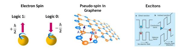
Figure 2: Electronic spins, pseudo-spins in graphene, and excitons are some of the novel state variables studied for beyond-CMOS logic devices [40], [41].
