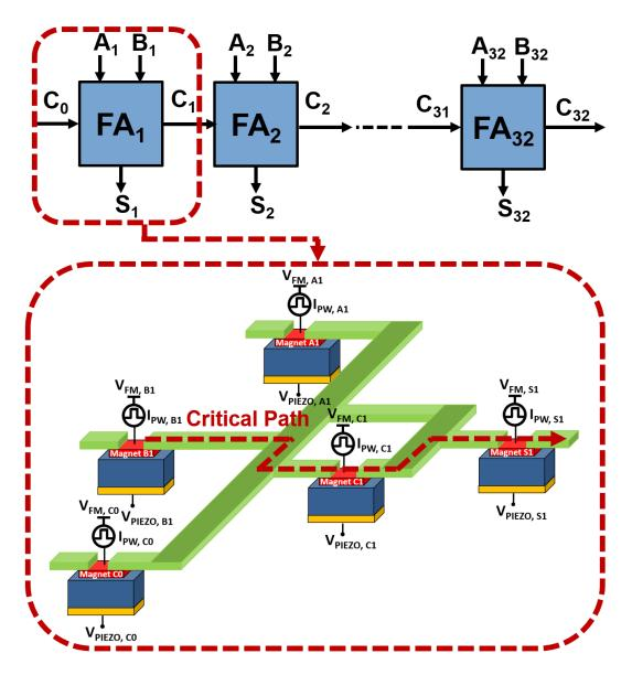
Figure 53: 32-bit ripple carry adder consisted of 32 full adders (FAs). Inside each full adder, two MA-ASLs form the critical path. Inside the 32-bit adder, carry bits must propagate through the critical path, comprised of 64 magnets.
