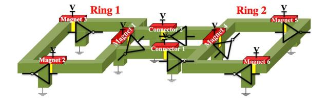
Figure 21: (a) Two metallic channels are connecting two ASL ring oscillators to form the ASL coupled oscillator. The oscillation of the two rings will be coupled to each other if the oscillation frequencies of two oscillation loops are close to each other.
