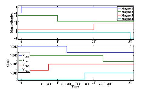
Figure 45: Clocking schemes used to minimize the energy dissipation of the ASL repeaters. Clocks are on  $\alpha$ T before and after the mean switching time to cancel the potential impact of thermal noise.  $\alpha$  is assumed to be 25% in the simulations.
