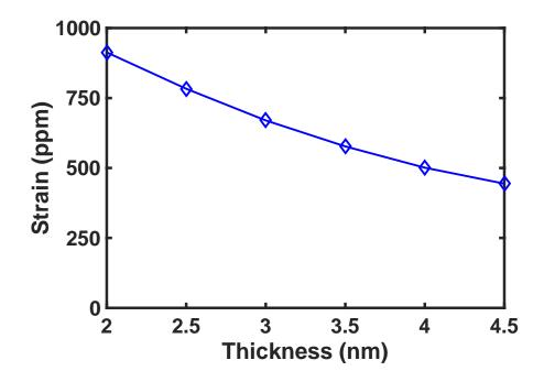
Figure 58: Transferred strain to the magnet vs the thickness of the Pt layer between the piezoelectric and magnetic layers.
