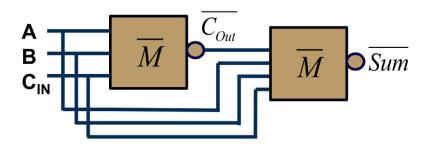
Figure 18: Implementation of a full adder using two majority-not gates.
