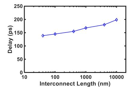
Figure 75: Switching delay vs interconnect length. The increase in delay with length compared to that of an ASL is significantly smaller. Thus, MASO circuits do not require repeaters even for interconnects as long as 10  $\mu m$ .
