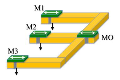
Figure 24: An ASL Majority gate with three inputs. The three input magnets, M1, M2 and M3 are connected to the output magnet, MO, using three metallic channels.
