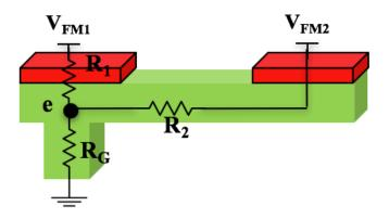
Figure 42: ASL gate modeled by a star network of resistors for calculating the electrical current passing through the input magnet.
