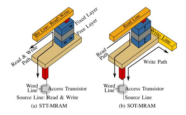
Figure 79: Bit-cell for STT-MRAM and SOT-MRAM [223].
