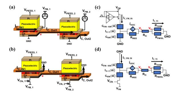
Figure 70: Two driver circuits are proposed for MASO repeaters in (a) and (b), and their corresponding circuit models are represented in (c) and (d).
