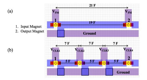
Figure 41: (a) Layout of an ASL gate that transfers spin signals through a metallic interconnect, (b) layout of ASL gates in a cascaded structure, which is a solution to transfer spin signals in long interconnects. The meaning of colors is defined in [33].
