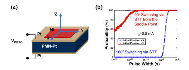
Figure 7: (a) 90° magnetostrictive switching is experimentally demonstrated [64]. (b) Compared to 180° magnetization reversal via applying STT, 90° switching of a magnet via STT from the saddle-point of energy profile is demonstrated to be two orders of magnitude more delay and energy efficient [65].
