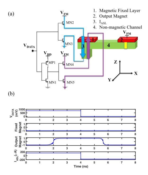
Figure 39: Electrical signal to spin signal transducer: (a) schematics of the transducer. (b) Input signal (V<sub>DATA</sub>), which switches the polarity of the voltage applied to the fixed magnet, which switches the output magnet accordingly. The orientation of the output magnet follows the input signal with a delay of 1.6 ns and 2.0 ns for high-to-low and low-to-high switching.
