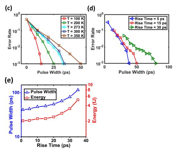
Figure 56: (a) Definition of pulse skew. (b) The required pulse width to reach to an error rate of  $10^{-3}$  for various pulse skews in an MA-ASL inverter. Positive compared to negative pulse skew, has more impact on increasing pulse width. Error rate vs pulse width for various (c) temperatures and (d) rise times. (e) The pulse width and energy to reach to an error rate of  $10^{-3}$  for various rise times. The pulse skew is assumed to be -5 ps in Figures (c), (d), and (e) [148].
