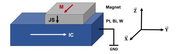
Figure 67: Spin-Hall effect in a hybrid heavy metallic/magnetic structure [180].
