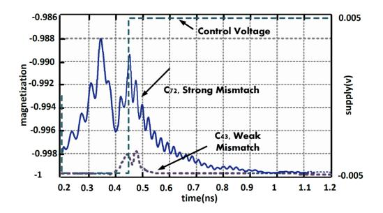
Figure 38: For the cases of mismatch in clusters, magnets will not switch and the initial magnetization does not change. The y-axis shows a range from -1.002 to -0.998 in contrast with Figure 37 in which the range is from -1 to 1.
