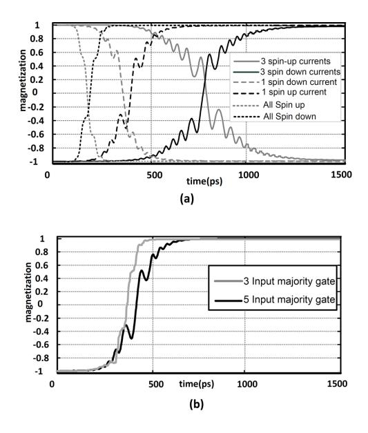
Figure 25: (a) Switching transient response for different scenarios of input magnetization in a majority gate with 5 inputs. (b) Switching transition comparison of majority gates with three and five inputs. In this comparison, the input magnetization of magnets of three input gates are the same. For the gate with five inputs, four inputs have similar magnetization and the net spin current is equal to the other gate. The applied voltage on magnets in these simulations is -5 mV.
