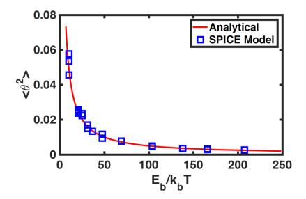
Figure 13: To validate the SPICE model of the thermal noise, the derived average value of the thermal noise over time of the SPICE model, is compared to that of the analytical solution. SPICE results match with analytical results.
