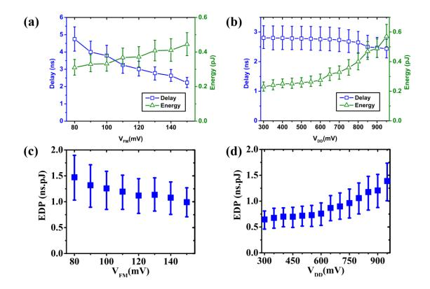
Figure 48: Delay and energy dissipation variations vs. (a) the voltage applied to the magnets  $(V_{FM})$  and (b) the supply voltage  $(V_{DD})$ . Energy-delay product (EDP) variations vs. (c)  $V_{FM}$  and (d)  $V_{DD}$ . The interconnect must operate at the lowest  $V_{DD}$  and the highest  $V_{FM}$  voltage values without reaching its breakdown current density
