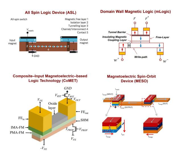
Figure 3: Several spintronic devices are proposed, such as the all spin logic (ASL) device [27], the composite-input magnetoelectric-based logic technology (COMET)
