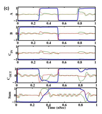
Figure 19: (a) Schematics and (b) layout of the ASL full adder. (c) The transient response of an ASL full-adder. The blue color represents the magnetization orientation in the x-direction and the green and red colors are representing magnetization in the y and z directions.
