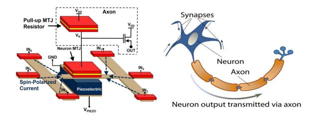
Figure 62: (a) Proposed MA-ASL neuron, shown with six inputs. The net spin current in the interconnect applies STT to the free layer of the neuron MTJ in timing with the piezoelectric clock, switching the orientation of the neuron output [166]. (b) Biological neural network [162].
