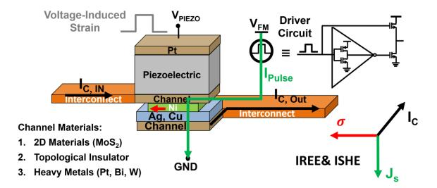
Figure 69: Schematics of proposed magnetostriction-assisted spin-orbit (MASO) logic device. The read and write operations are done in three phases. To write data into the magnet, first, magnetostrictive switching is employed to rotate the magnetization by  $90^{\circ}$ . Second, SHE is applied to perform the second  $90^{\circ}$  of switching. In the third phase of operation, the stored information is converted into the direction of the output charge current that can drive the next stage.
