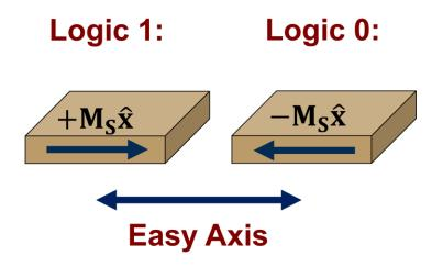
Figure 5: Binary information is stored as the magnetization orientation along the two stable directions along the easy axis of the magnet.
