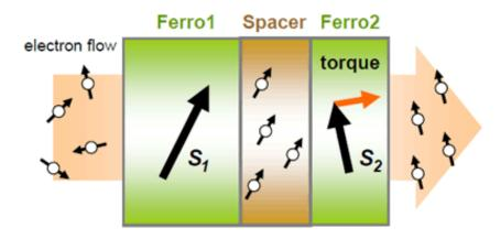
Figure 6: Spin-transfer torque explained in a spin valve [60].
