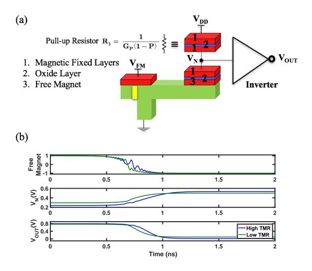
Figure 40: Spin signal to electrical signal transducer: (a) schematics of the transducer. (b) the changes in the orientation of the free magnet are translated into changes in electrical voltage on the node  $V_N$ . The inverter provides a full swing between the ground and supply voltages at accordingly. Simulations are done for two TMR values of 131% (low TMR) and 355 % (high TMR).
