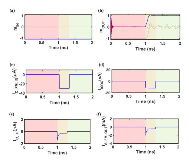
Figure 71: Transient response of the MASO device. The orientations of the input and output magnets are shown in (a) and (b), respectively. The supply current is shown in (c), and the charge current generated beneath the magnetic layer is shown in (d). Some of the generated charge current passes through the TI layer below the output magnet as shown in (e), which applies an effective transverse spin current shown in (f) to the output magnet.
