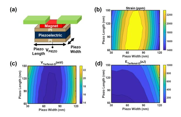
Figure 59: Analysis on the transferred strain vs geometrical dimensions of the piezoelectric layer. (a) definition of piezoelectric dimensions. (b) Transferred strain at a constant  $V_{PIEZO}$  voltage of 100 mV. The required (c) voltage and (d) energy to transfer a net strain of 1200 ppm.
