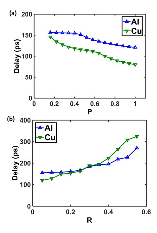
Figure 16 : (a) Delay versus specularity parameter, P, for an 80 nm long channel. Grain boundary scattering parameter, R, is assumed to be 0.2 (b) Delay versus grain boundary reflection probability for an 80nm long channel. The specularity parameter, P, is assumed to be 0 [96]–[99].
