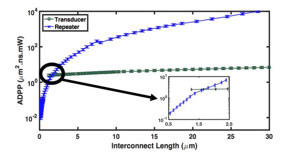
Figure 47: Area-delay-power product (ADPP) is a measure that takes delay, power dissipation, and area into account. Although the proposed interconnect has larger area overhead, its advantage in terms of energy enables it to outperform ASL repeaters for lengths longer than  $1.6 \mu m$ .
