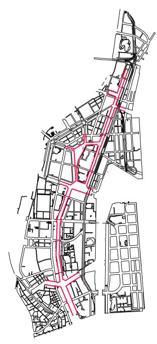
Proposed Stormwater Retention System
