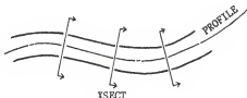
Figure 3.13 - Example of a road shown in plan depicting the orientation of sections generated by PROFILE and XSECT.
