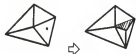
Figure 4.4 - Subdividing a triangular facet into three smaller facets through point insertion using the TIN model.
