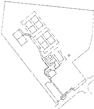
Graph H.11 - Plan view of Timbercreek II layout used to verify plot accuracy before three-dimensionally superimposing the layout on proposed topography.
