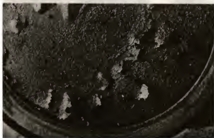
Figure 11. Top of Combustion Chamber after 200 hours Operation on Biomass Gas. (Top)
