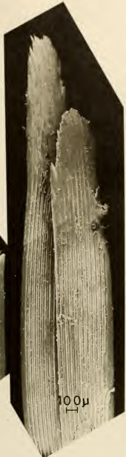
Figure 18: Synthetic Turf Fiber after 1000 Clock Hours of Weathering and 9000 Abrasion Cycles
