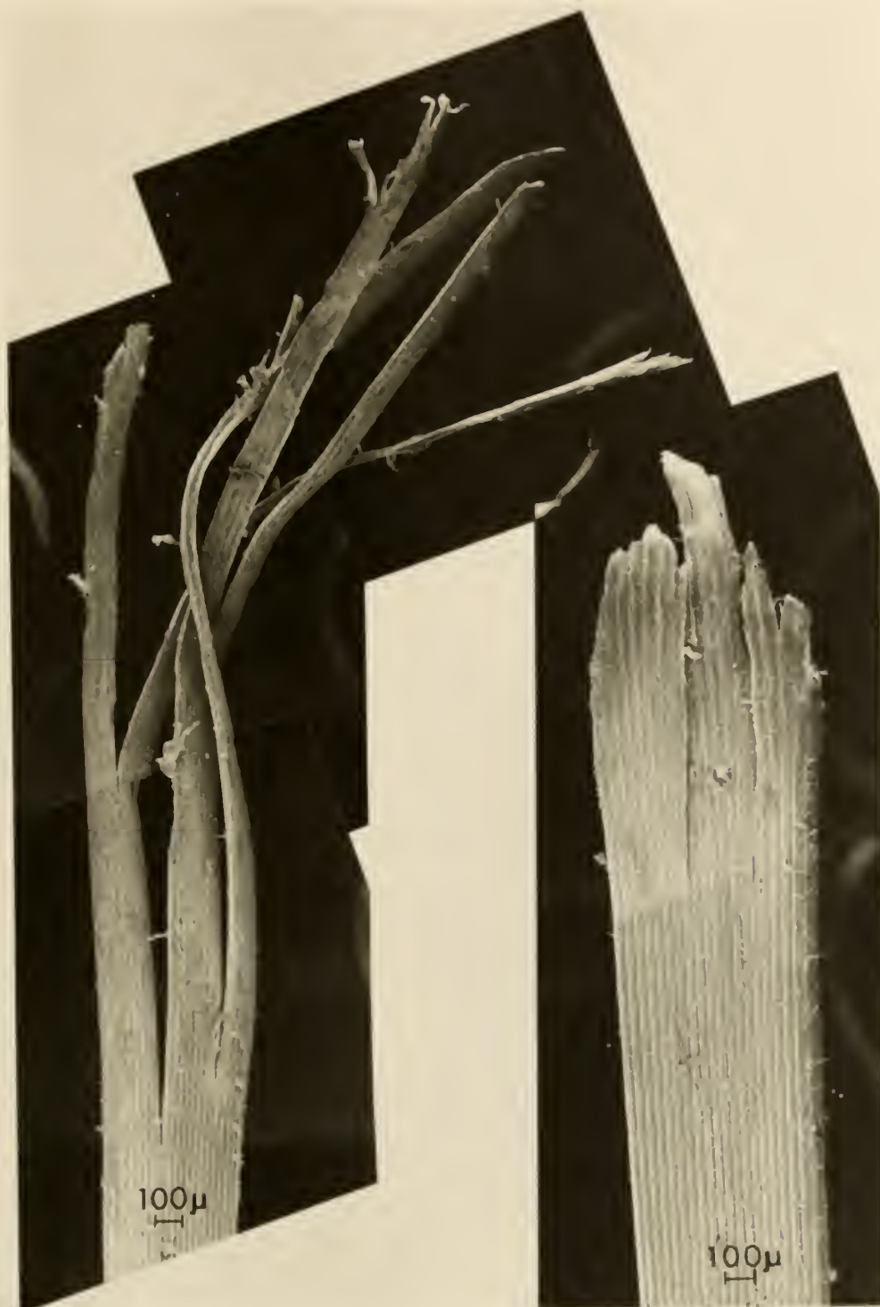
Figure 24: Synthetic Turf Fiber after 3500 Clock Hours of Weathering and 6000 Abrasion Cycles
