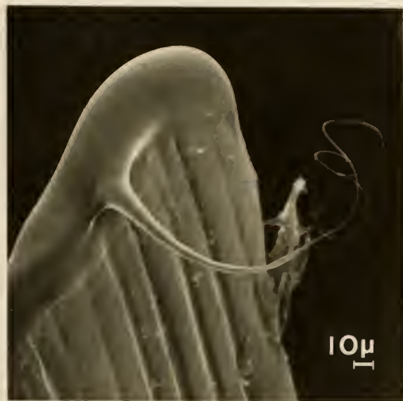
Figure 34: Synthetic Turf Fiber after 2000 Clock Hours of Weathering and 4000 Abrasion Cycles
