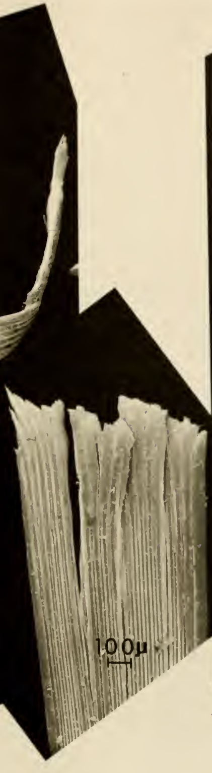
Figure 17: Synthetic Turf Fiber after 1000 Clock Hours of Weathering and 8000 Abrasion Cycles
