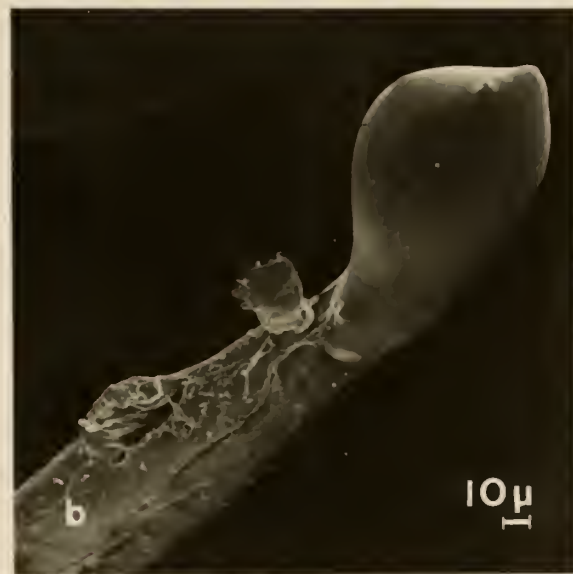
Figure 35: Synthetic Turf Fiber after 2000 Clock Hours of Weathering and 10000 Abrasion Cycles
