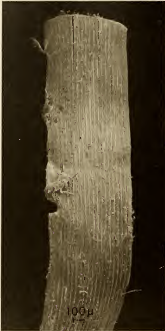
Figure 14: Synthetic Turf Fiber after 500 Clock Hours of Weathering and 1000 Abrasion Cycles
