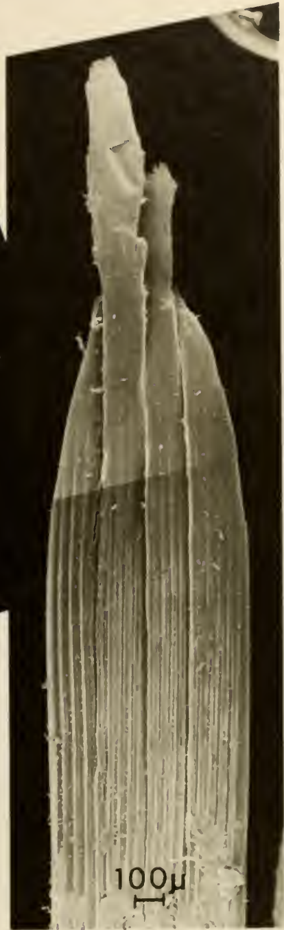
Figure 28: Synthetic Turf Fiber after 4000 Clock Hours of Weathering and 7000 Abrasion Cycles
