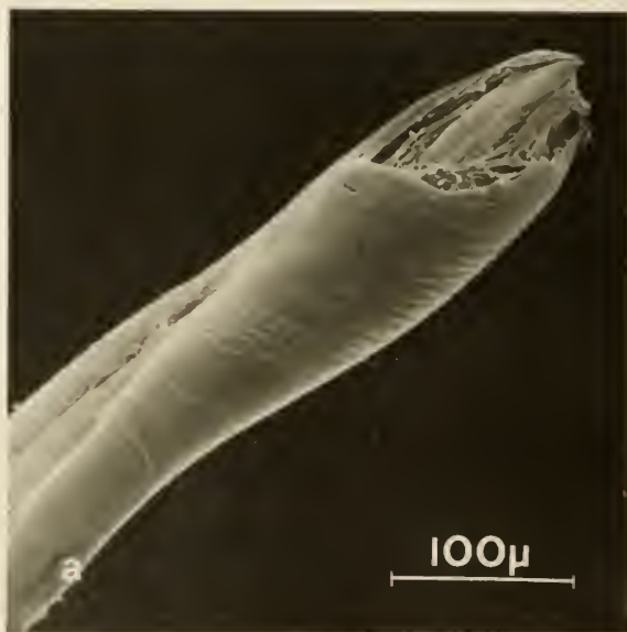
Figure 35: Synthetic Turf Fiber after 2000 Clock Hours of Weathering and 10000 Abrasion Cycles
