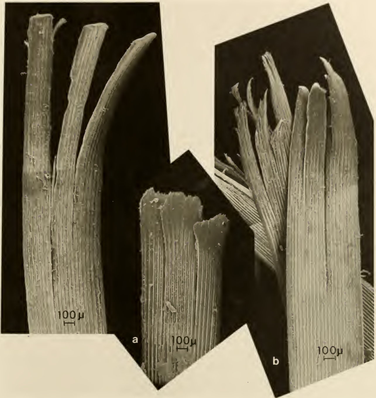
Figure 20: Synthetic Turf Fiber after 2000 Clock Hours of Weathering and 5000 Abrasion Cycles
