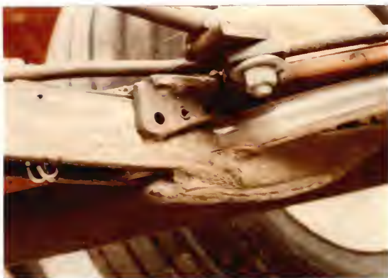
Figure 20. Angle iron shield to protect seed tube.
