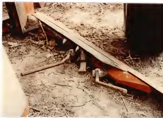
Figure 22. Seed delivery tubes with compaction openers removed.
