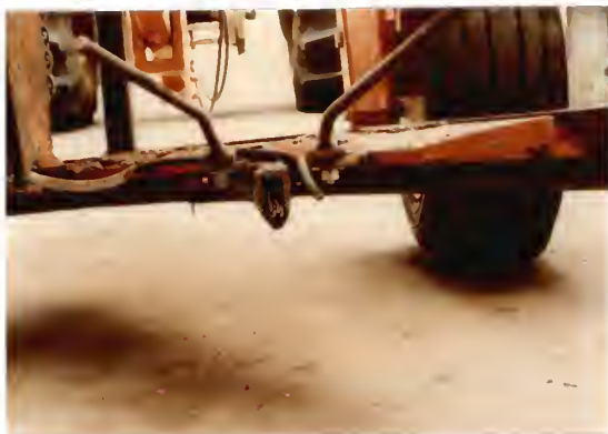
Figure 11. Compaction opener, fertilizer delivery tube, and cover control rods.
