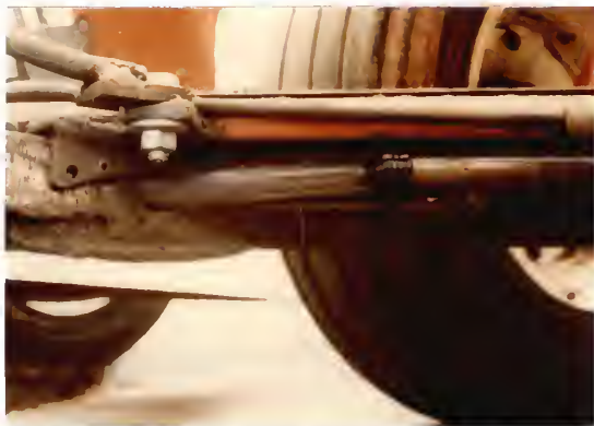
Figure 18. Compaction opener and side entry of seed delivery tube.
