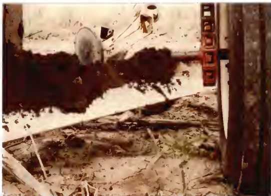
Figure 19. Soil buildup below blade caused by compaction openers.
