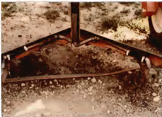
Figure 21. Extended blade with seed tubes mounted above the blade support and entering the compaction opener from above.
