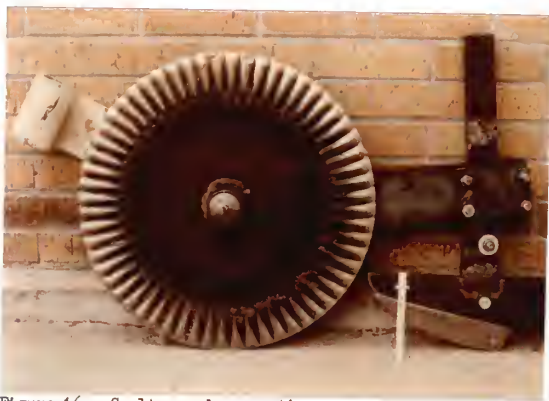
Figure 16. Coultter and compaction runner opener.
