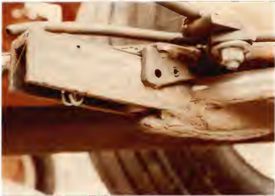
Figure 9. Compaction opener mounted below V-blade.
