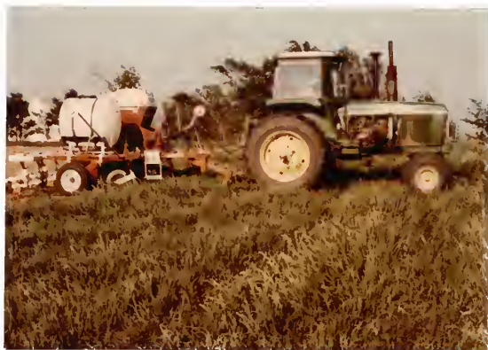
- Figure 35. Testing power requirements of undercutter planter with instrumented John Deere 4630 tractor.
