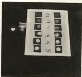
Fig. 4. Chart showing the range of partial sheet bleaching.
