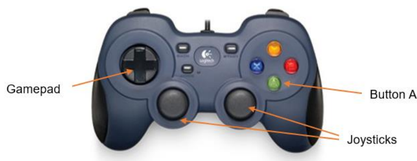
Figure 8. Analog Controller Used as User Interface in Unity
