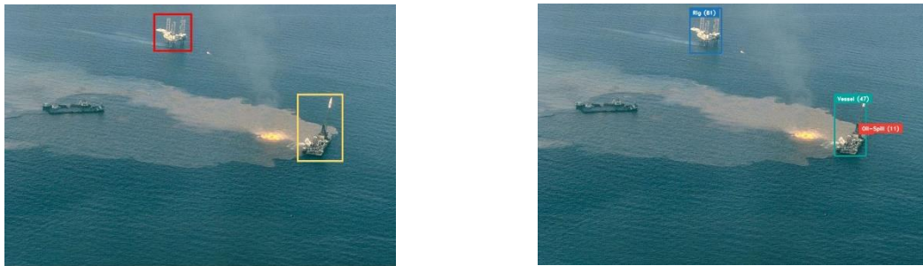
Figure 29 Sample Image from the Test Dataset (Left) and Corresponding Detected Image by YOLOv3 (Right).
