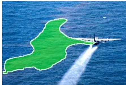
Figure 47 Example of False Positive Due to Low Contrast between Oil Spill and Background.
